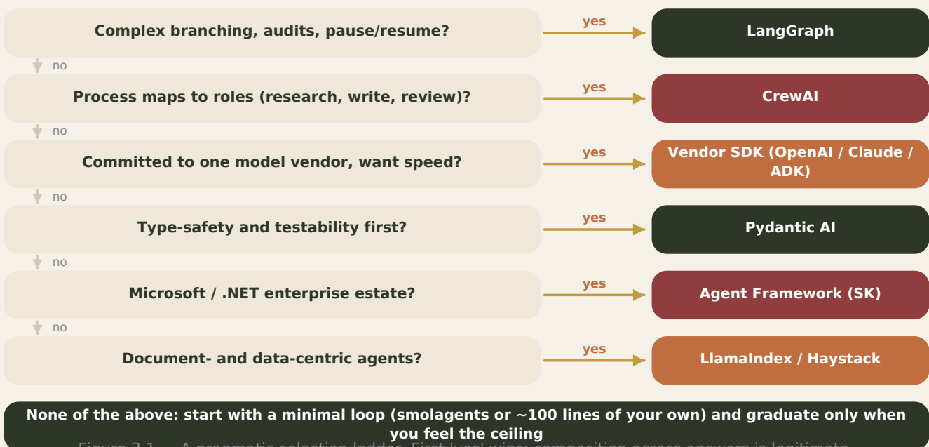
Figure 3.1 — A pragmatic selection ladder. First 'yes' wins; composition across answers is legitimate.
